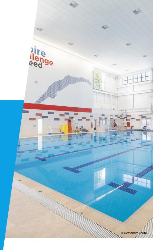
HYGENA Aquatec is the ideal solution for high-humidity areas of up to 100% RH. It offers excellent sound absorption, and its washable, which makes it the perfect solution for hygiene and healthcare environments. The surface is washable and anti-microbial.
